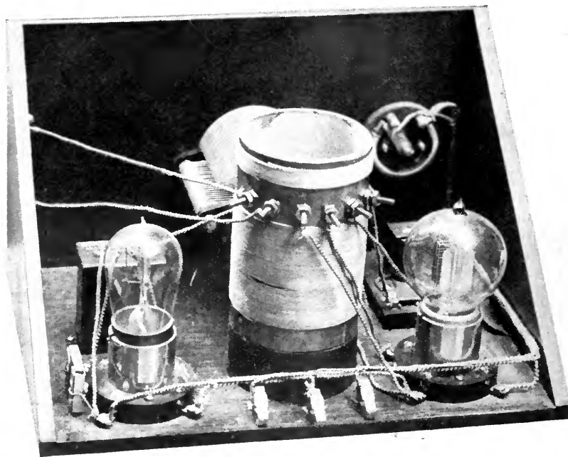
FIG. 7 Experimental type of wavemeter oscillator. The large coil is used as an oscillator, the smaller coil is a modulator creating an audible note. This type is not as convenient to construct as that shown in Figs. 5 and 6. This oscillator is made for use on a measuring bridge. It covers a wavelength band of 200 to 600 meters
